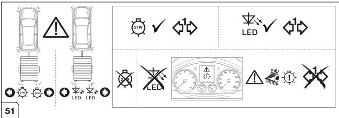
The following light functions for the trailer are not **supported** by all towing vehicles **with DRL circuit:**
